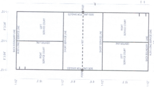
DIAGRAM E. Court which can only be used for singles play. ** Optional testing marks.
