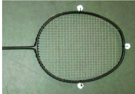
Figure 2.5: Attachment of reflective markers to racket head using zip-ties.
