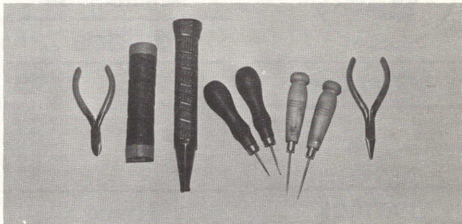
The Patch Kit (Lt. to Rt.) Duck Billed Pliers, Awls, Rollers, Diagonals
