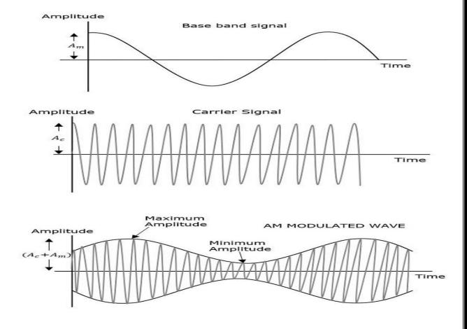
The first figure shows the modulating wave, which is the message signal. The next one is the carrier wave, which is a high frequency signal and contains no information. While, the last one is the resultant modulated wave
