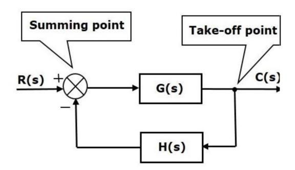
The block diagram above consists of two blocks having transfer functions G(s) and H(s). It is also having one summing point and one take-off point. Arrows indicate the direction of the flow of signals.
