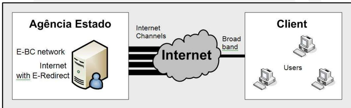
The client-server connection is kept during all the service utilization time, however, in the case of loss of connection with the server, the client software automatically will make a new connection with other **e-bc** server.
